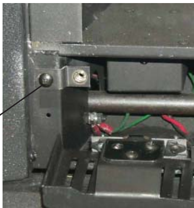
Secure bracket with screw.
